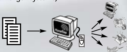
1. PhoneTree reads your call list and call job specifications from your PC. 2. PhoneTree sends your messages (automatically, or at your command).
